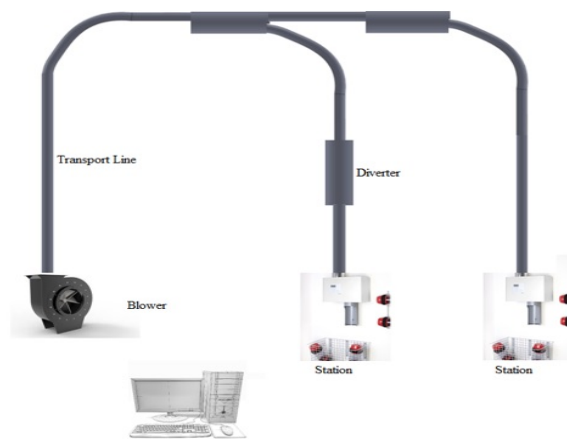
Figure 1. Basic hospital pneumatic system diagram.
