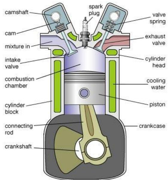
**Figure 1(a).** Internal combustion engine (courtesy: <http://mechanicalengineeringnotebook.com>)
