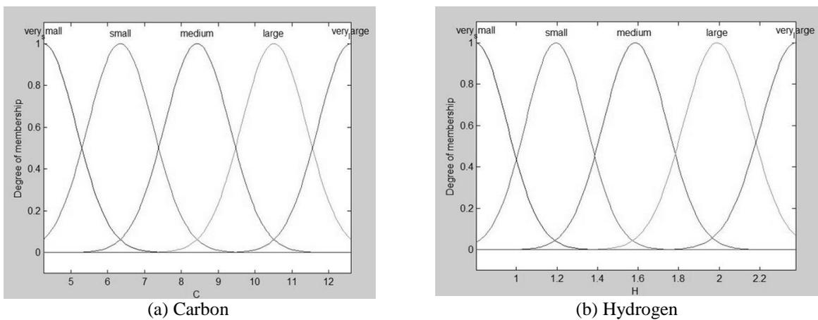
Figure 5. Input membership function for training data (Detector)
