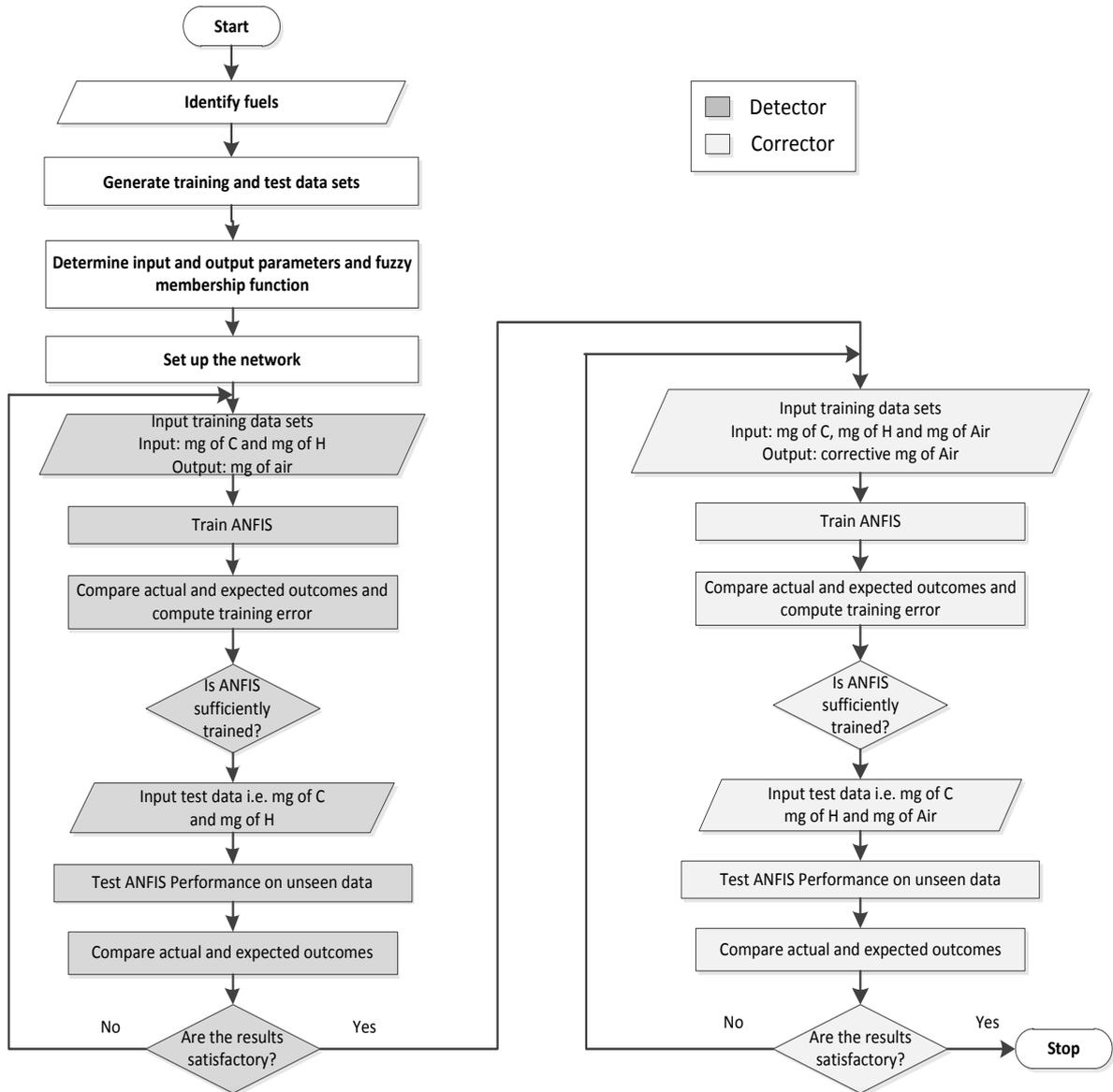
Figure 4. Flowchart for separate training and testing for detector and corrector of model
