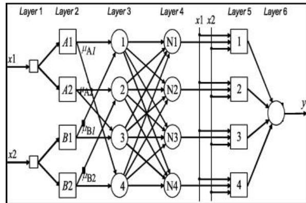
Figure 2. Six-layered ANFIS architecture
