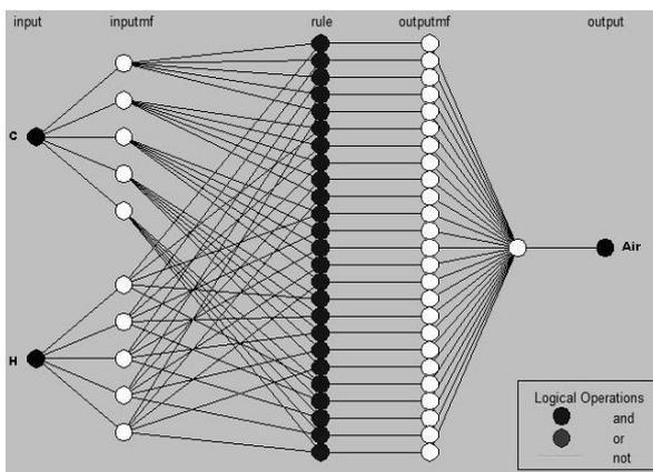
Figure 8. ANFIS structure (Detector)
