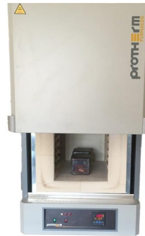
Figure 1. Heat treatment furnace where boriding process is performed.
