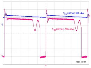
$\label{eq:Figure 10. Voltage stress on switching component (V_{DS})} and snubber circuit voltage (V_{SN}).$
