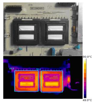
**Figure 7.** Thermal analysis under 25°C ambient temperature [14]
