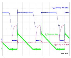
$\label{eq:stress} \begin{array}{l} \mbox{Figure 12. Voltage stress on switching component (V_{DS}), \\ \mbox{switching component trigger voltage (V_g) and current on} \\ \mbox{PFC converter diode (I_g)} \end{array}$
