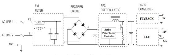
Figure 1. Sub-blocks of the PSU design
