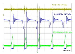
Figure 8. Flyback converter output voltage ( $V_{OUT}$ ), voltage stress on switching component ( $V_{DS}$ ) and primary current ( $I_{PRI}$ )
