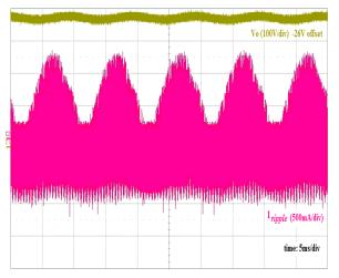
Figure 13. Voltage on output capacitor (V<sub>0</sub>) and ripple current ( $I_{ripple}$ )
