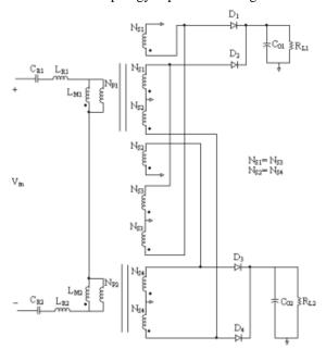
Figure 3. LLC resonant converter topology [14]
