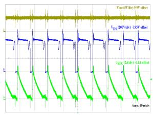
Figure 9. Flyback converter output voltage ( $V_{OUT}$ ), voltage stress on switching component ( $V_{DS}$ ) and secondary current ( $I_{SEC}$ )
