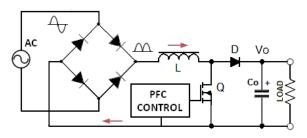
Figure 4. Boost type PFC converter topology
