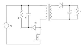
Figure 2. Flyback converter topology
