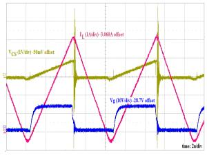
Figure 11. CrM PFC converter bobbin current (I<sub>L</sub>), voltage on current measurement node (V<sub>CS</sub>) and switching component trigger voltage (V<sub>g</sub>)
